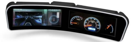
Capacitive Touch Panels with Large Curved Cover Glass
