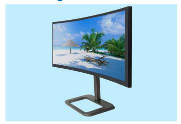
SMK Corporation has developed the "Wing Touch MM" capacitive touch panel that uses a copper mesh sensor for large and curved surfaces found on medium and large sized displays.
