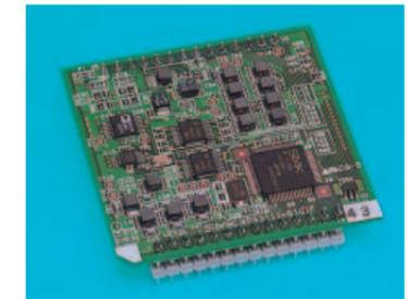
DS-SS Modulation/ Demodulation Engine for PLC
