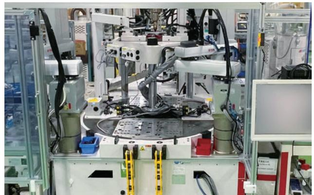
Production facilities for automotive connectors using SCARA robots
