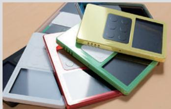
Sensor unit using hybrid technology of energy harvesting and wireless power transfer.
