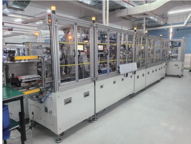
Remote control assembly automation machine using 6-axis robots (Dongguan Factory, China)
