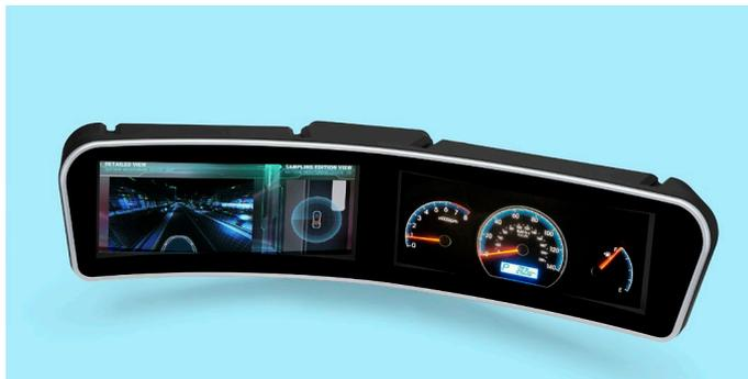
SMK Corporation has developed the "CapDuo Touch-S", a combination of thin glass capacitive touch sensors with a large curved cover glass, ideal for automotive displays.
