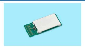
SMK Corporation has developed dual-mode Bluetooth modules "BT801" and "BT801-AP2" (collectively called "BT801 Series") that support both Bluetooth Classic and Bluetooth Low Energy communications. The new series has the same shape and pin- and command-compatibility with the conventional BT401 Series, making it easy to replace them.
