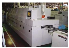
Lead-free reflow soldering machine
