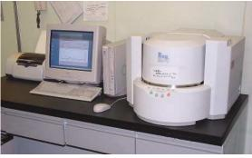
XRF spectrometer for heavy metals analysis
